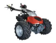
The CC 160 has a **23 hp** electric-boosted two-cylinder petrol engine. The driving speed can be ergonomically adjusted to your needs with the new ten-stage TipTronic.
